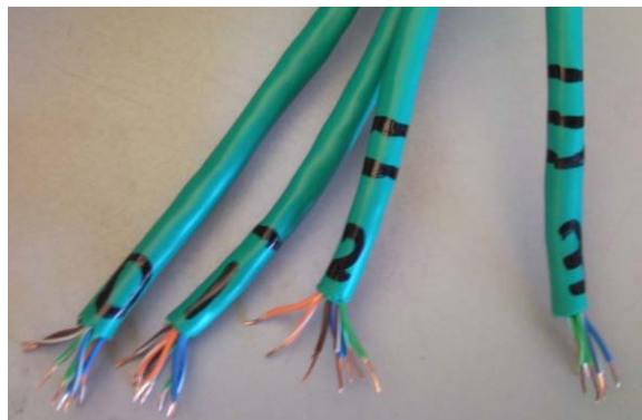
Figure 16.5 Four cables with a total of 32 individual wires provide the detector connections to each interface box.
