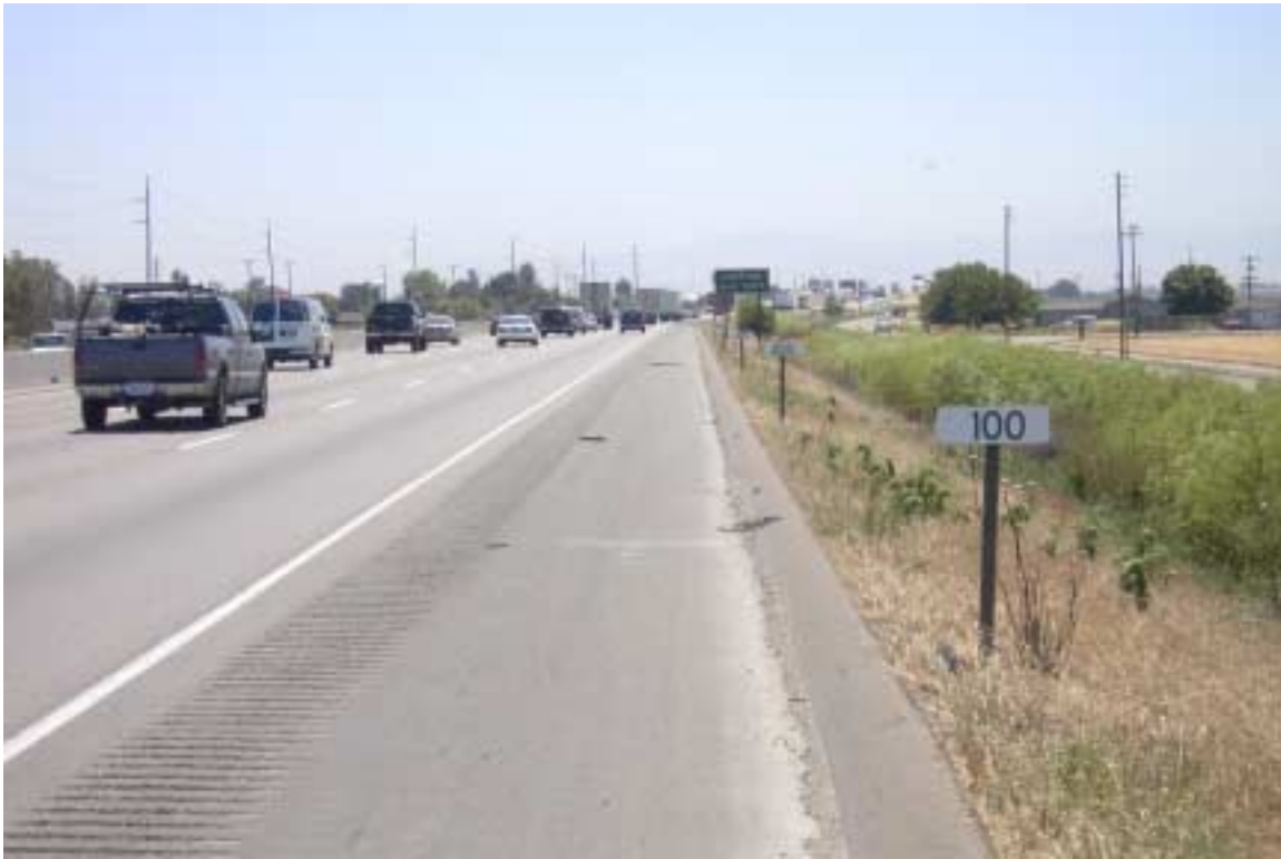
Figure 3.2.5.2. Visibility distance reference placards installed south of WS 4 by Caltrans District 10 personnel for manual verification of local visibility.
