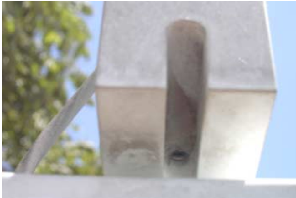
Figure 3.2.5.4. Day/night sensor blocked by spider egg sac.
