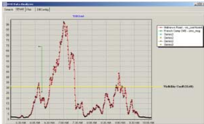
Figure 3.3.4.2. D10 Analyzer Screenshot, showing graphical depiction of fog over the course of an activation event, 11-07-04.
