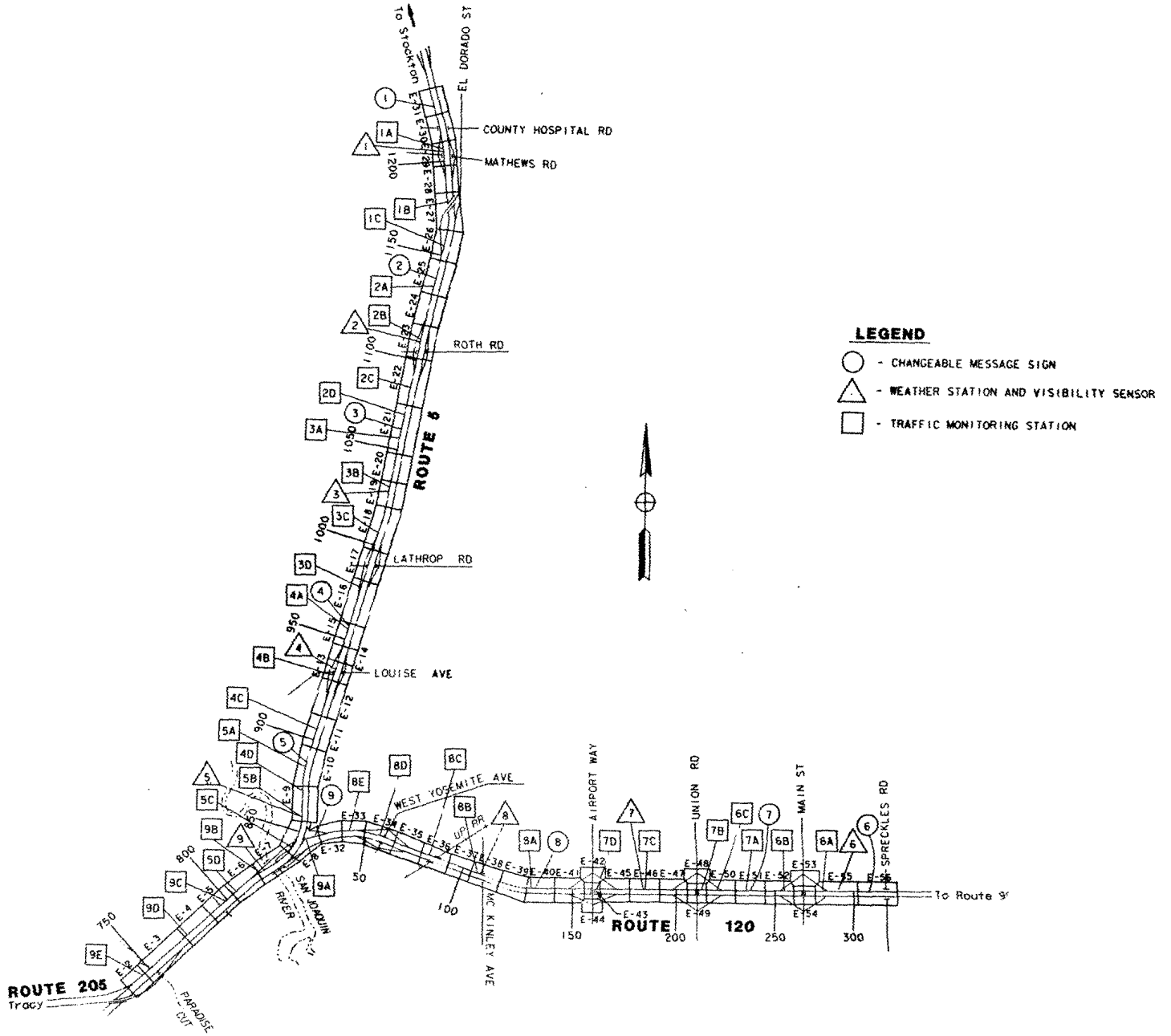
Figure 3.2.2.1. CAWS elements deployed on I-5 and SR-120. From Caltrans as-built drawings for CAWS project.
