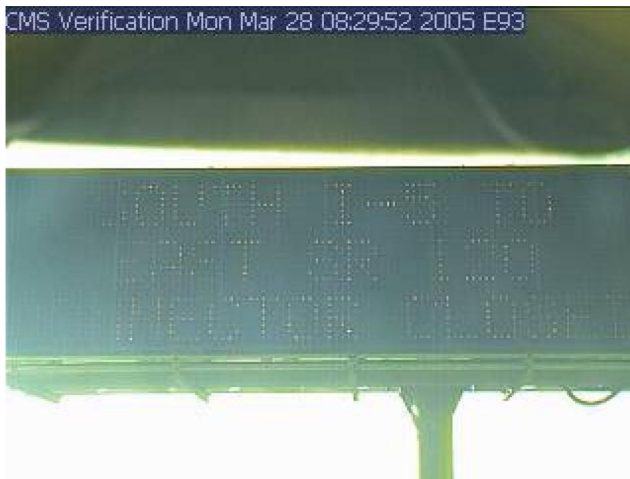
Figure 5.8.3.12. (Type S) camera image of CMS message during fog.
